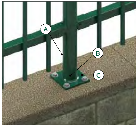
BASE PLATE Option of incorporating base plate to install the posts on concrete walls and gates with a height > 2m00. Dimensions of the plate 120x120x8mm. A. Post B. Wall plate C. Anchor
